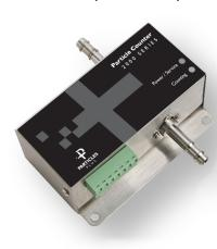
The Particles Plus® 2301-1 Remote Particle Counter measures 0.5  $\mu$ m and 5.0  $\mu$ m with a flow rate of 0.1 CFM (2.83 LPM). Integration is easy into a real-time monitoring or building management system via Modbus RTU. The 2501 models are the smallest remote particle counters on the market and have easy mounting options. The Particles Plus® 2501 units comply with ISO 21501-4 and include a 1 year limited warranty.
